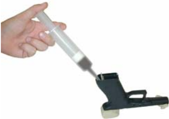
Fill the grip recess with bedding compound.
