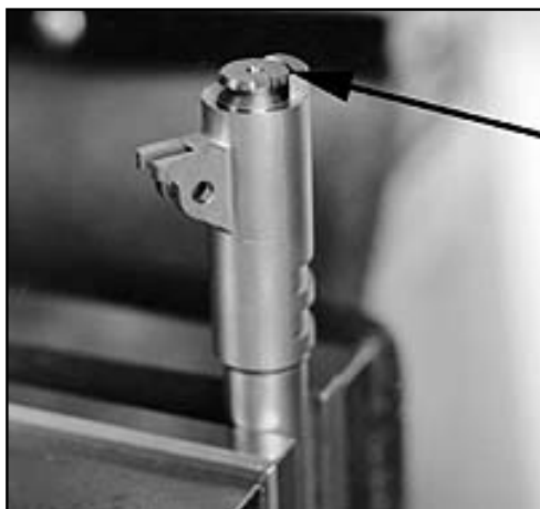
Small step at arrow shows amount of headspace (+.005”) with a Clymer GO gauge placed in the chamber of a .45 ACP, 1911 Auto barrel
