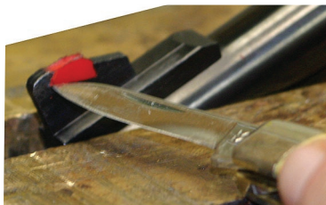
Gently scrape the edges clean with a pocket knife
