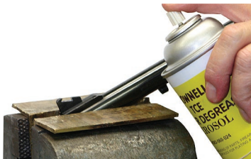
Clean thoroughly with TCE
