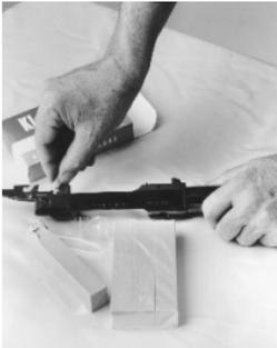
openings, pits, recesses and deep machine marks in the barreled action, recoil lug and triggerguard/floorplate with modeling clay. Smooth with scraper to keep all surfaces flush. Make certain the recoil lug, or any other projection, is not wider at the bottom than at the top. A reverse taper like that can mechanically lock the barreled action into the stock once surrounded by **ACRAGLAS GEL**.
