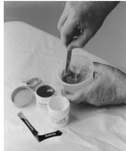
**Time/Temperature Note:** At 72°-75° F, you have approximately 25 minutes working time before your **ACRAGLAS GEL** becomes too stiff to use and give a suitable bonding between epoxy and stock. At higher room temperatures the
