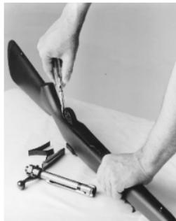
of the barreled action with a soft rubber mallet and try again. Proceed with the firm, slow lifting once the stock and barreled action begin to separate. If you still can't get the barreled action out, don't force it! Give our Tech Support staff a call and we'll help.
