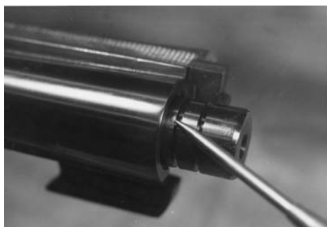
Classic example of short chamber. After thorough cleaning, chamber will not accept gauge to full 2¾" depth. This particular chamber measured 2⅝" prior to rechambering.
