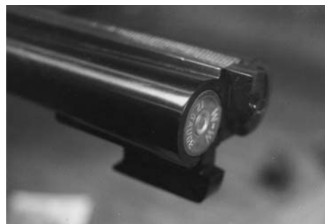
The same chamber as shown at left, still prior to rechambering, easily accepts an unfired 2¾" shell. However, when fired, this shell will protrude into the forcing cone area, causing excessive pressures, recoil and damage to the gun. Following these photos, this gun was rechambered to 2¾".
