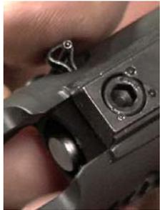
1. Pull the firing pin retainer pin out of the carrier and remove the firing pin.
