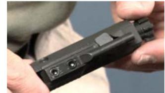
7. Insert the cam pin so the long flat surface is parallel to the carrier. Rotate the cam pin ¼ turn.
