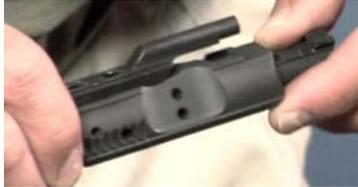
2. Push the bolt to the rear of the carrier and rotate the cam pin so the long flat surface runs parallel with the carrier. Remove the cam pin and pull the bolt out of the carrier.
