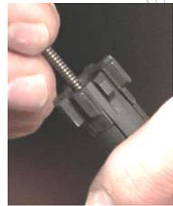
5. Unscrew the ram and remove the ejector and spring.
