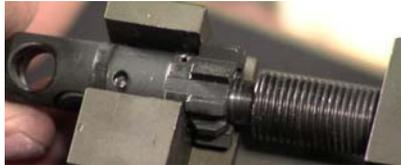
4. Use the number 1 roll pin punch drive out the ejector roll pin.
