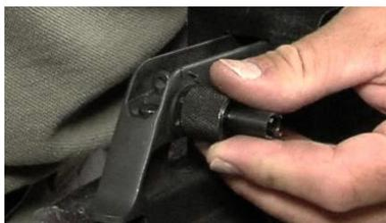
Test the function of the sight by first flipping up and down the rear aperture. It should snap forward and back with some resistance.
