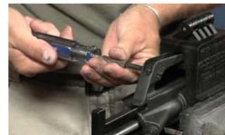
3. Install the sight windage screw from the left hand side and thread it into the sight until the sight is in the middle of the handle and the screw sticks out completely on the other side with the hole facing upward.
