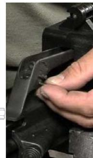
6. Use your needle nose pliers to keep pressure on the drum and roll pin. Turn the windage screw from the left hand side until you can align the hole in the screw with the hole in the windage drum. Once aligned, use the pliers to push in the roll pin.
