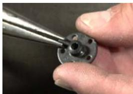
5. Place the sight detent spring and detent into hole under the screw and place the windage drum onto the end of the screw with the pin facing up and lined up with the pin hole on the windage screw.
