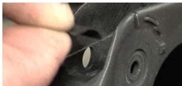
2. Place the flat sight spring and the rear sight aperture onto the carry handle. making sure the small sight aperture is up and facing you with the large aperture laying down.
