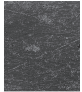
The same barrel at 100X magnification after FLEX HONE ing. Note removal of most of the "peaks".
