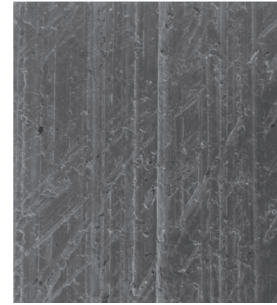
After FLEX HONEing , scratches are replaced by cross hatch (100X).
