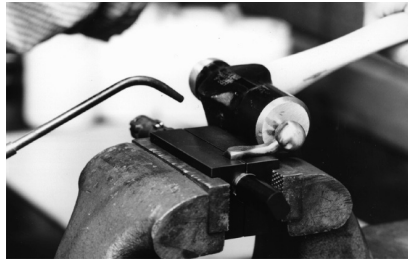
Sweeping the bolt handle back about 15° from vertical.
