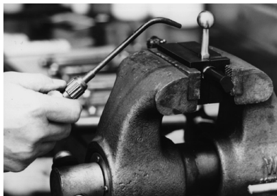
Applying heat to the standard bolt handle.
