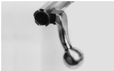
Cutout at rear of Small Ring Mauser bolt, after cleanup.
