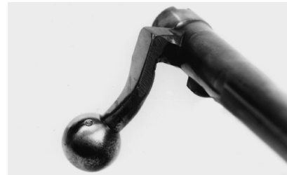
Front view of finished M-98 bolt knob.
