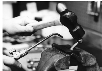
Initial bolt forging with a ballpeen hammer.
