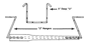
welding rod, being sure to remove any plating or covering on the rod. The bottom leg of the "Z" slips into the barrel, and the top leg makes a convenient handle. The top and bottom limb should be about 3" to 4" long; the center leg at least 7" to 8" long.
