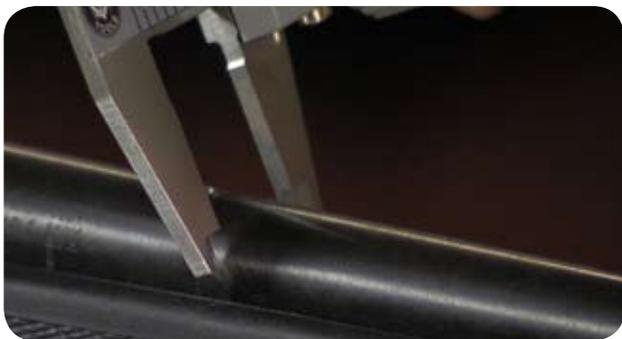
Barrel Dia. Measurement At Rear Sight .820"
