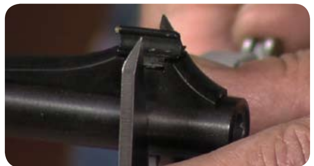
Barrel Dia. Measured At Front Sight .596" .596'' \div 2 = .298''
