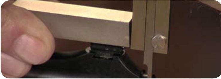
Measure the height of the existing front sight. Add the height of the front sight to its corresponding bore-center-line to top-of-barrel figure to obtain the distance between bore-center-line and line of sight.
