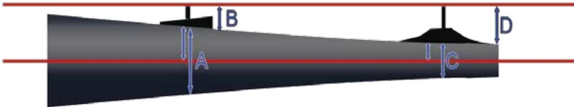
**The distance from the bore-center-line – shown running through A and C – to the line of sight – shown at the tops of the sights -- must be the same approximate distance or height at each sight location. The rear sight has an adjustment range and you should use the middle of the range as your starting point for measurements or to determine the correct sight for the rear sight.**
