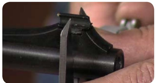
Barrel Dia. Measured At Front Sight .596"
