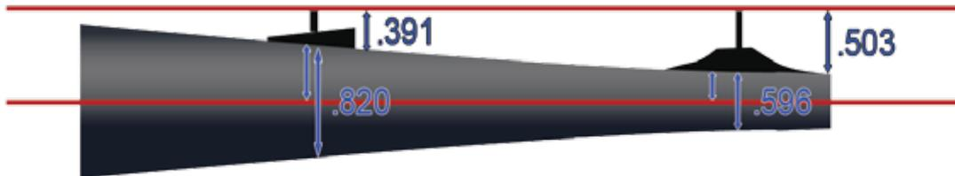
One half barrel diameter at front sight plus front sight height will give height of sight line above bore-center- line. Height of sight line above bore-center-line minus one half barrel diameter at rear sight will give rear sight height
