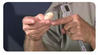
When you get the scope at the height you want it, measure the thickness of the clay which will give you the total height of the base and ring combined. Take this measurement, consult the Brownells catalog or web site to determine what base/ring combination you need.
