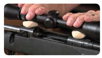
Place your scope on top of the balls, making sure your eye relief is correct and press down on the scope while making sure it is level.
