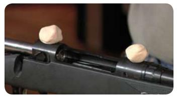
You simply take a little modeling clay and roll it into a couple of balls (maybe about ¾" in diameter or larger if needed) and set one between the front scope mount holes and the other between the rear scope mount holes.
